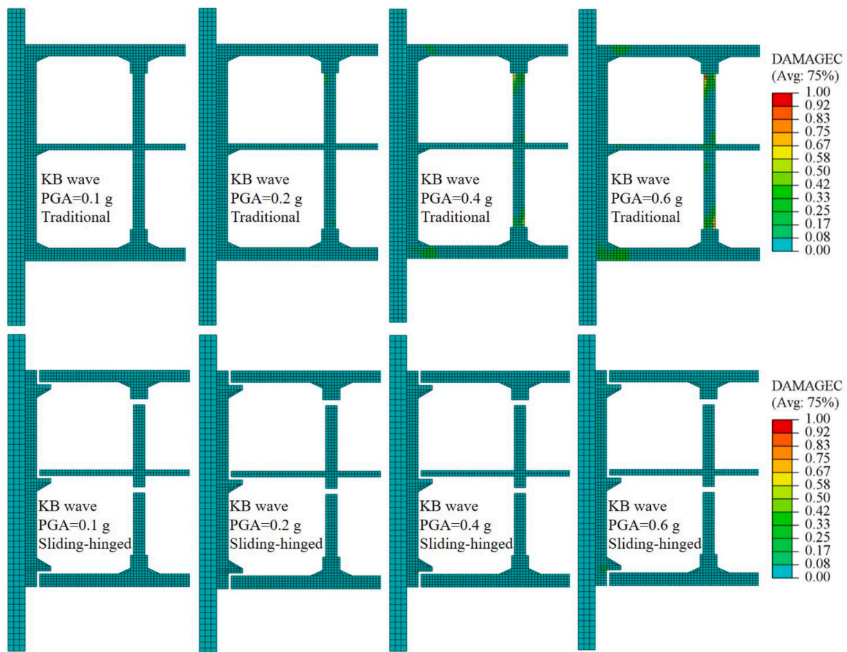
Fig. 16. Compression damage nephogram of the station with innovative design. KB wave.
