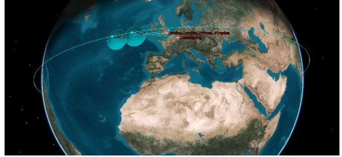
Fig. 4: Sample LEO orbit with two following Cubesats designed in STK (500 km altitude and 52 degrees of inclination).
