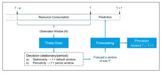
Figure 1: Diagram of the ThetaScan Algorithm
