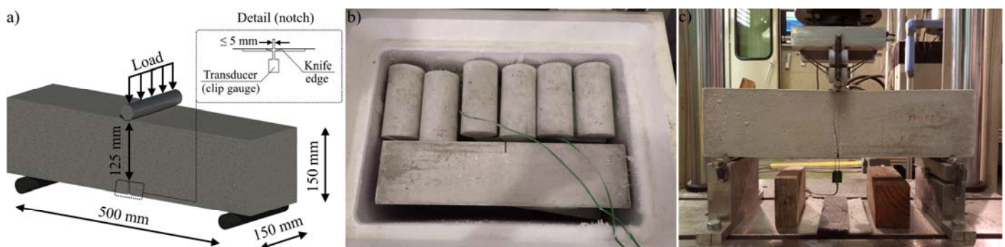
Figure 2. (a) 3PBT setup; (b) freezing procedure and temperature monitoring; (c) 3PBT at −30 °C.
