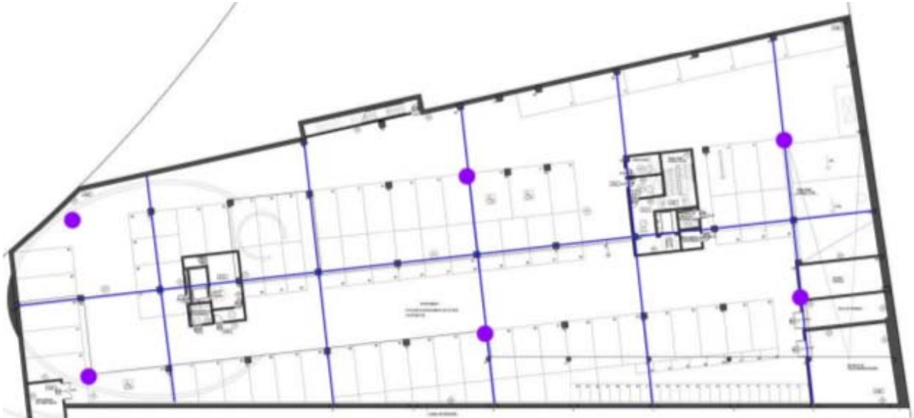
Fig. 7 Example of medium intensity sensorisation in the Neapolis building.
