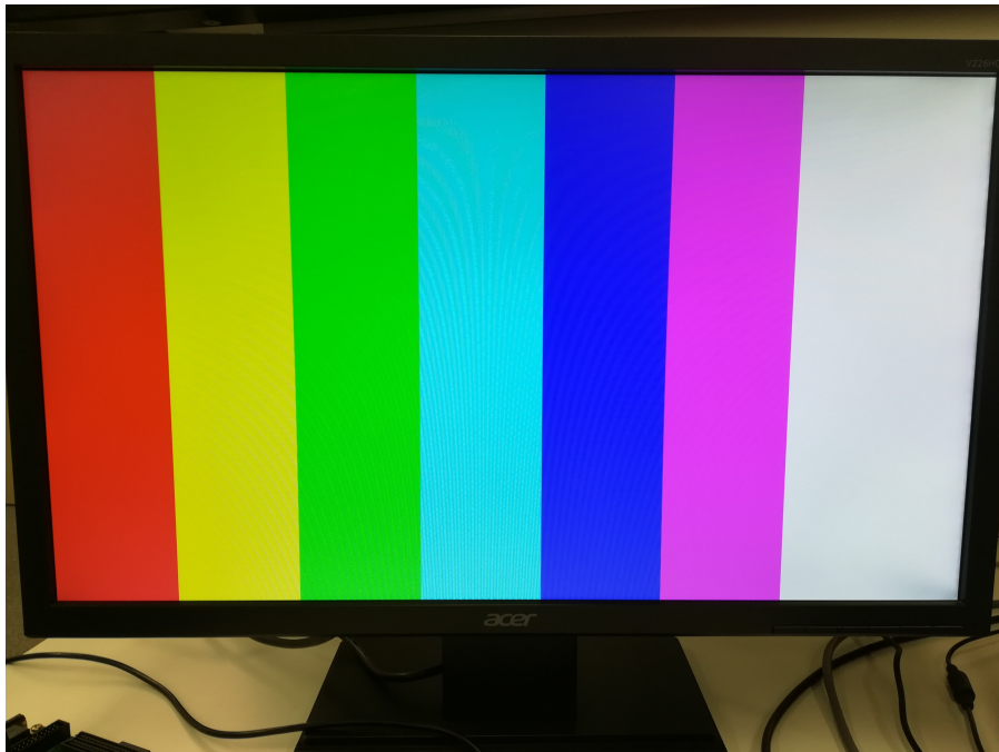
Figure 27: Result screen of the HDMI test.
