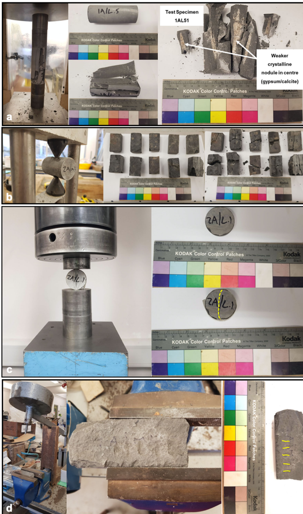
Fig. 7 (a) UCS test; (b) Point Load test; (c) Brazilian test; and, (d) CERCHAR test configuration and post and pre-tested sample mudstone examples for each test
