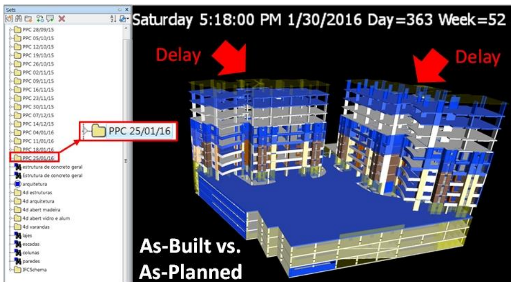
Figure 10 - Simultaneous as-built and as-planned visualization and analysis
