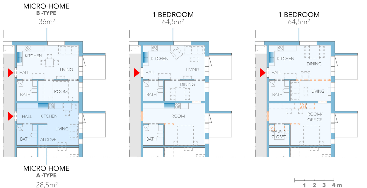
Figure 15 Illustration of the connectivity of a micro-home (A-Type) with a B-type micro-home, creating one larger 1-bedroom unit; note that a large part of the indoor space will remain poorly lit due to the deep-plan design of especially the A-Type micro-home. On the left-hand side is the original plan with two micro-homes, and in the middle is the connection of the micro-homes into a 1-bedroom apartment without disconnection of services; the right-most image indicates disconnection of services.
