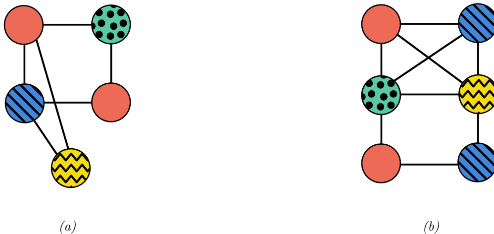
Figure 3.3: Examples of valid graph colourings. The graph in (a) is the same as in Figure 3.1a but the colouring here is not optimal as the graph could also be coloured with only three colours. The colouring for (b) is optimal.
