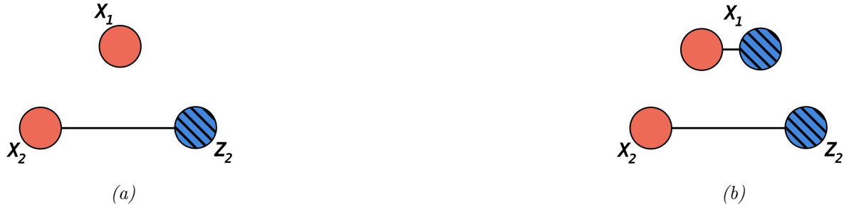
Figure 4.2: (a) The observables from Example 4.2 can be coloured with two colours. If X_1 requires two measurements while the other two need only one, this colouring would lead to three measurements. (b) If we assign a weight two for the X_1 vertex, we can find a multicolouring with two colours. This way, only two measurements are needed.
