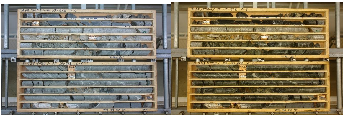
Fig. 23: Representative part of the KOMBAS unit taken from drill hole R318 (left dry, right wet). The boxes include some mafic volcanic rocks, while some felsic veins are visible (lower part of the lower box)
