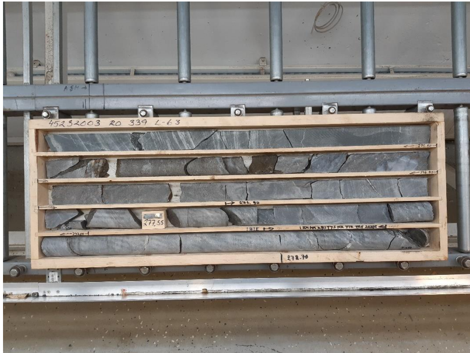
Figure 22: Representative part of the CALC1 unit, taken from drill hole R339 at the area of U-Pb sampling for sample R339. The schistosity of the rock is visible as well as some veinlets
