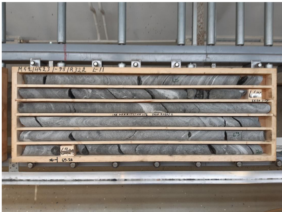
Fig. 25: Representative sample picture of the unit CALC3, taken from drill hole R322 at the depth of U-Pb sampling for the correspondent R332 sample. There are felsic volcanosedimentary rocks with visible schistosity and quartz veins penetrating them.
