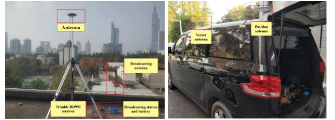
Fig. 5. RTK base station (left) and vehicular experiment (right).
