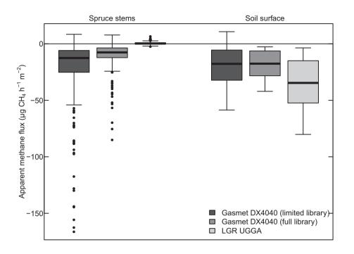
Fig. 1 Apparent CH<sub>4</sub> flux from soils and tree stems in a boreal forest stand, as measured using Fourier transform infrared (FTIR) spectroscopy (Gasmet DX4040) and laser absorption spectroscopy (LGR UGGA). Spectral deconvolution for FTIR was conducted with a full or limited spectral libraries. Figure taken from Kohl et al. (2019).
