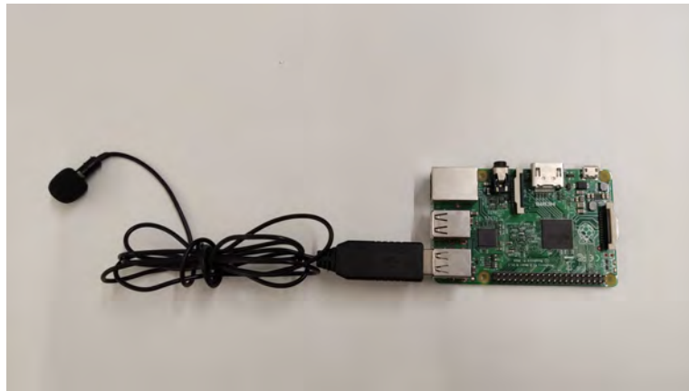
Figure II.2: Raspberry Pi Model 2B with USB microphone.
