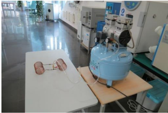
Fig. 4. Pressure Testing of the HCOHPs.
