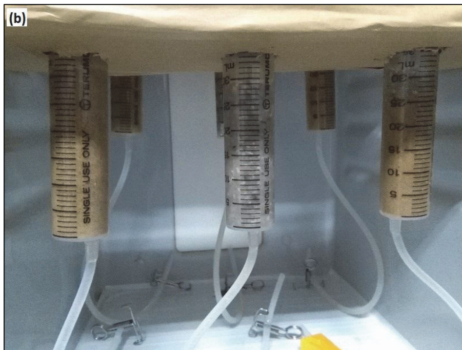
Figure 2: (a) Conceptual setup and (b) images of the syringe solidification of coarse- and fine-grained sand.
