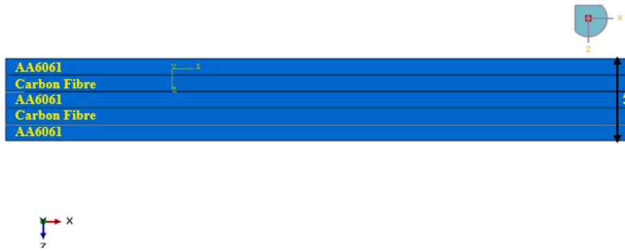
Fig. 10. Top view showing the individual components stacked together for Type-I FML.
