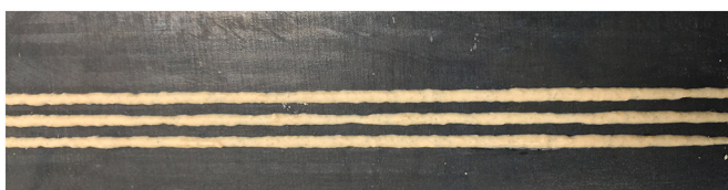
Fig. 3. – Extrudability assessment of mix design by printing three 200 mm lines.
