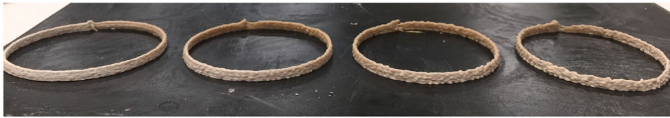
Fig. 7. – Printed objects with different surface quality due head distance issues (head distance increases from left to right).
