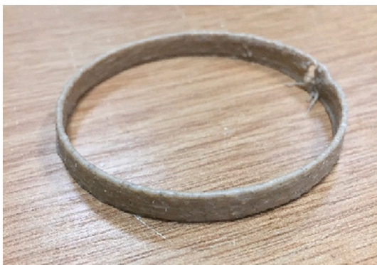
Fig. 5. – Ten-layer printed buildability ring.
