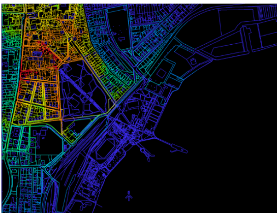
Figure 2. Space Syntax segment analysis – number of nodes - R = 800m / Keszthely. Melinda Bognár, 2020.
