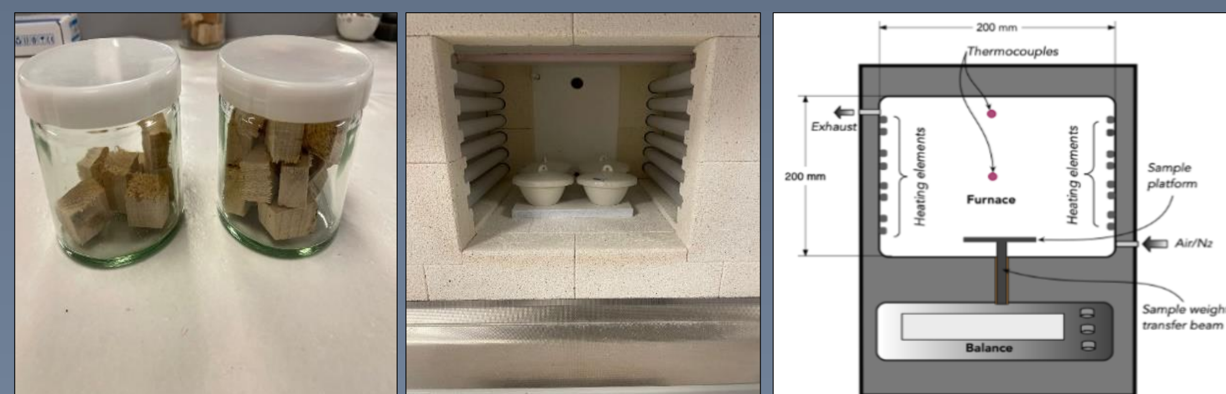
Sample position inside furnace (Precursor ~ 30 g).
