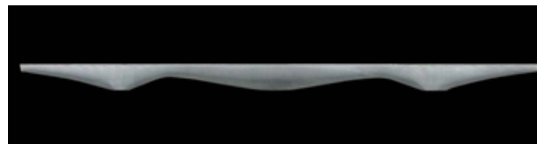
Figure 2.18: Concrete beam made with fabric formwork
