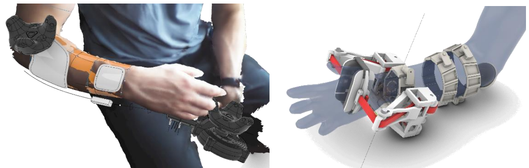
Figure 8. An initial arrangement of a linkage resulting in a rotation around a virtual axis aligned to the user’s wrist.
