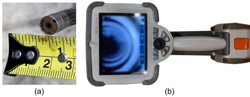
Fig. 1. (a) An inspection videoscope (header diameter 8.4 mm), with an embedded miniature camera. (b) The videoscope handheld, utilised to record inspection video footage.
