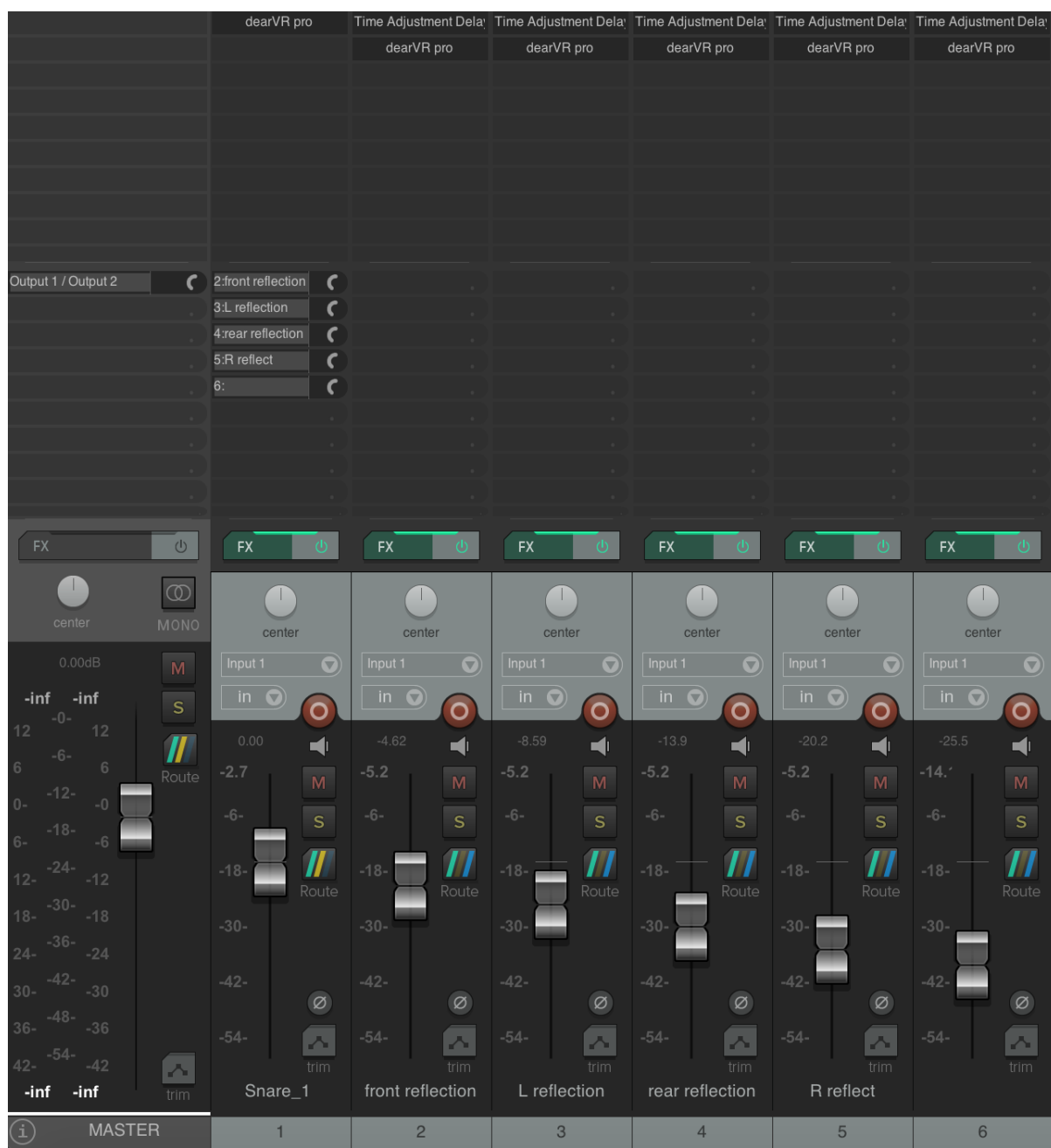
Figure 71: Reaper edit window showing the decreases in mix level (amplitude) of each delayed source.
