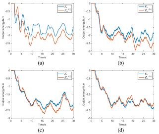
Fig. 6. Environmental input energies by using different controllers (a) Results of P+d control (b) Results of PD+d-like control with  $\eta_i = 1$  (c) Results of PD+d-like control with  $\eta_i = 0.7$  (d) Results of PD+d-like control with estimations of time delays and dynamics compensations
