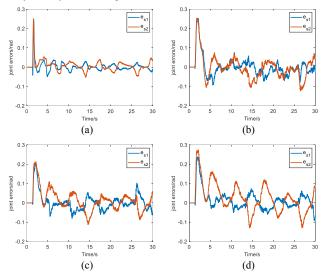
Fig. 5. Joint tracking errors using different controllers (a) Results of P+d control (b) Results of PD+d-like control with  $\eta_i = 1$  (c) Results of PD+d-like control with  $\eta_i = 0.7$  (d) Results of PD+d-like control with estimations of time delays and dynamics compensations
