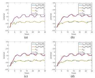
Fig. 4. Joint changes using different controllers (a) Results of PH control (b) Results of PD+d-like control with  $\eta_i = 1$  (c) Results of PD+d-like control with  $\eta_i = 0.7$  (d) Results of PD+d-like control with estimations of time delays and dynamics compensations
