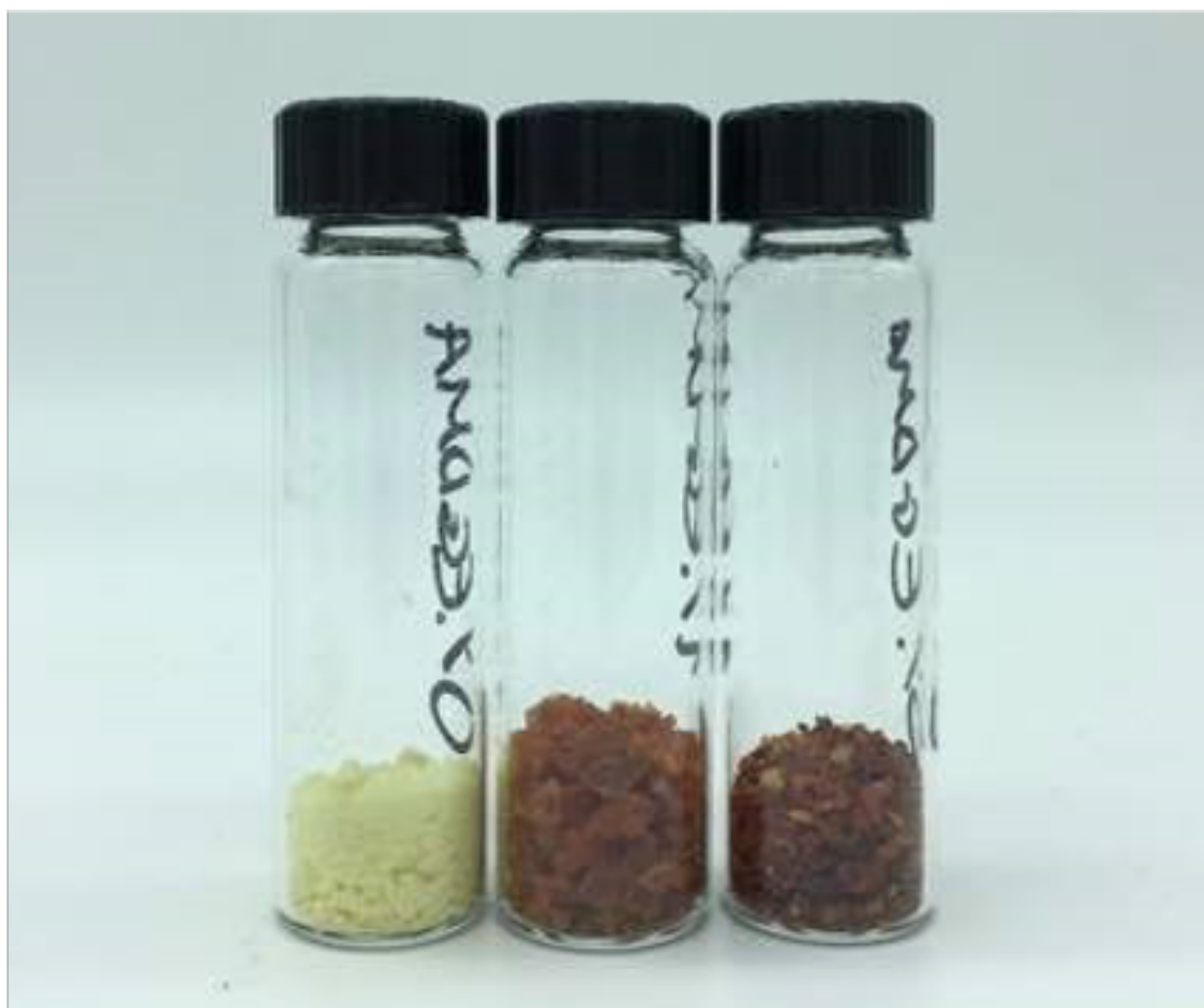
Figure 4.11: Photograph of produced polymer, S-EGDMA produced at different catalytic loadings: (left) 0 wt% (middle) 1 wt% (right) 5 wt%
