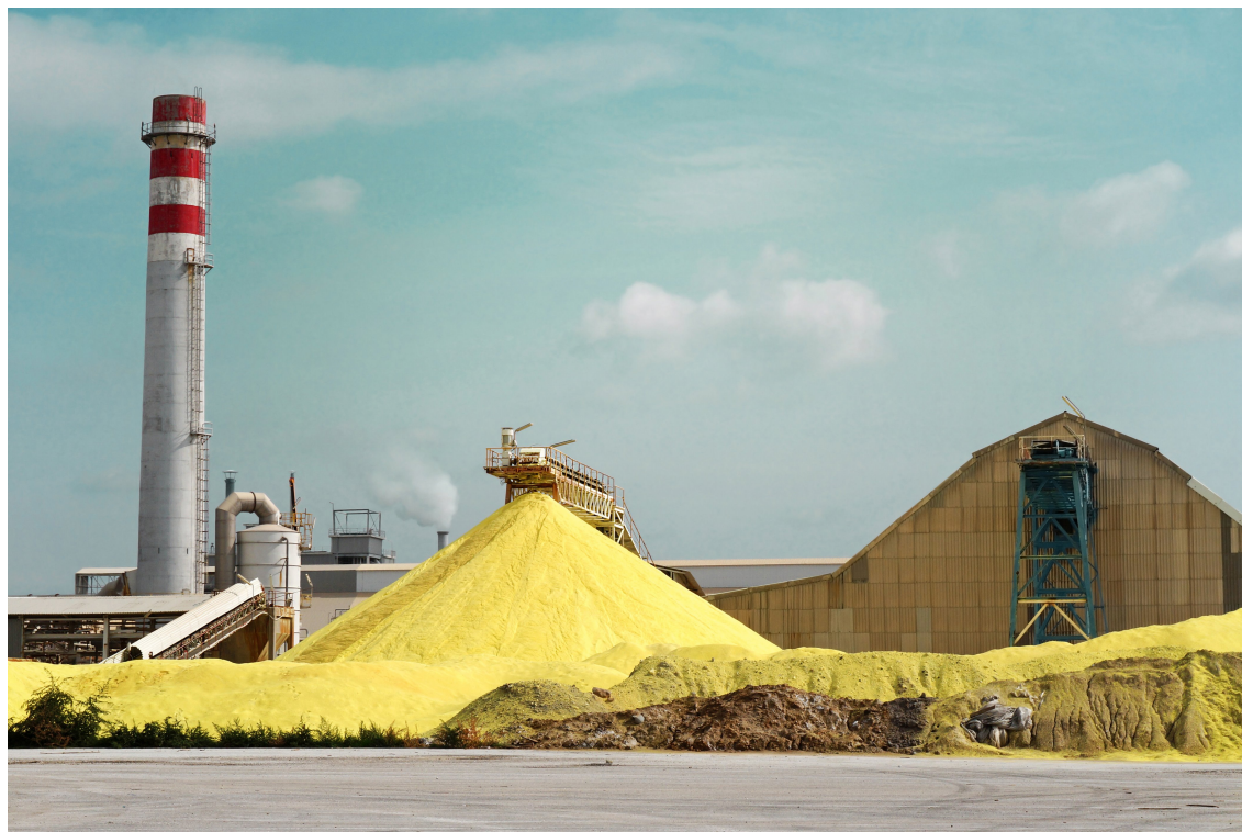
Figure 2.1: A monolithic pile of sulfur, resultant of the hydrodesulfurisation process. Located outside the Alberta oil sands, Canada
