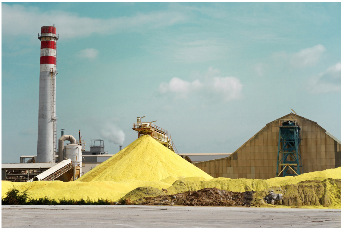
Figure 1.1: A large monolithic pile of elemental sulfur that is stored out on the Alberta oil sands, CA
