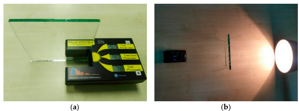
Figure 3. (a) EDTM-SS2450 instrument to measure the solar spectrum; (b) EDTM-SP2065 instrument to measure transmission power.
