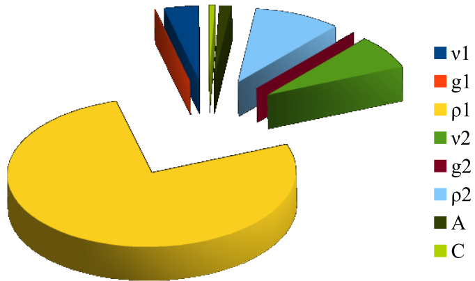
Figure 6.12 Proportional sensitivity of element with maximum second failure criterion to uncertain parameters
