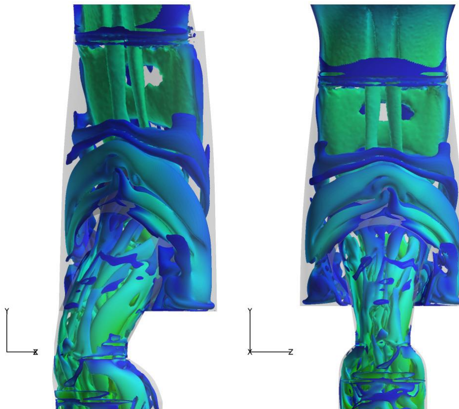
Figure 4.1.16 Iso-surface of Q-criterion colored by velocity magnitude, 10 l/min. Anterior and oblique (45°) of the pharynx and larynx from right to left. The geometry is in gray
