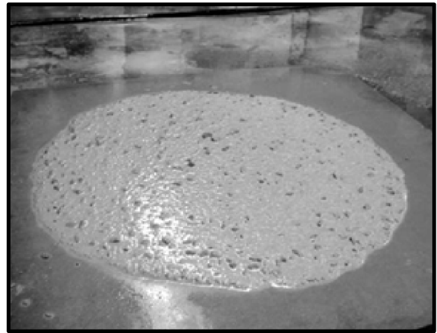
VSI = 2 – A slight mortar halo # 0.5 in.(# 10 mm) and/or aggregate pile in the of the concrete mass
