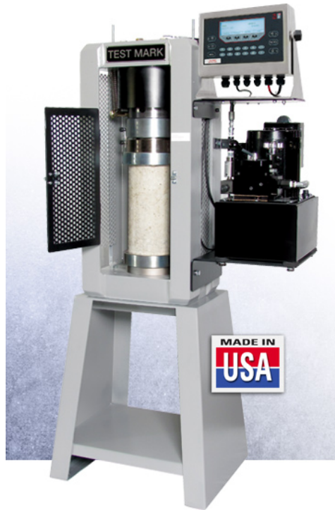
Figure 3.11 Compressive Strength Test
