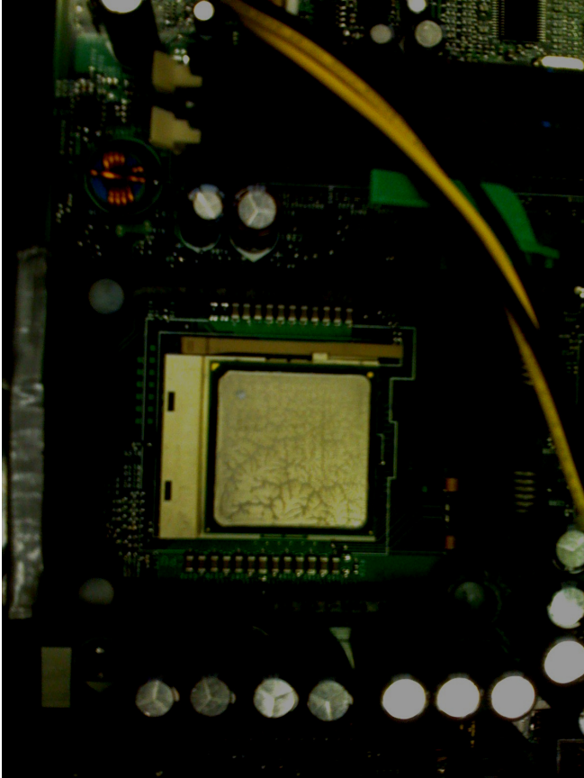
Figure 3.17 (c) – Pattern formations on the processor after the heat sink was taken out
