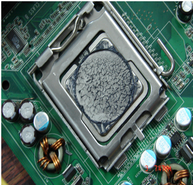
Figure 3.17 (a) – Pattern formations on the processor after the heat sink was taken out
