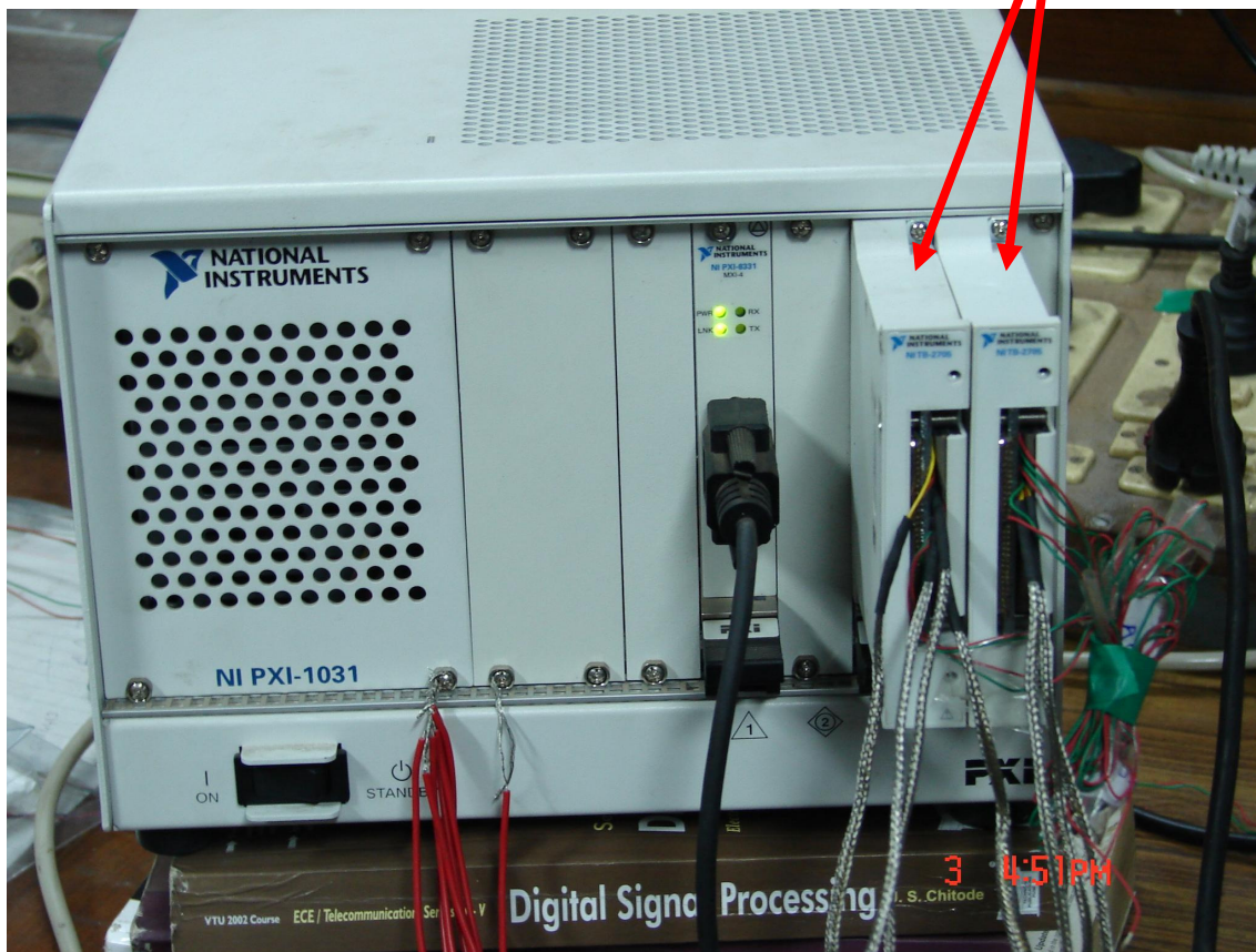
3.12 – NI PXI 1031, with two 4 channel NI-TB 2705 DAQ cards.
