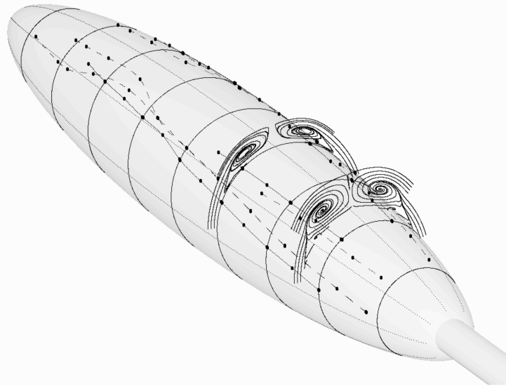
Figure 4.4: Experimental Data Showing Vortices Along the Major Axis of the Prolate Spheroid – Simpson’s experimental solution data showing vortices along the major axis of the prolate spheroid at x/L = 0.600 and x/L = 0.772 as well as velocity streamlines.
