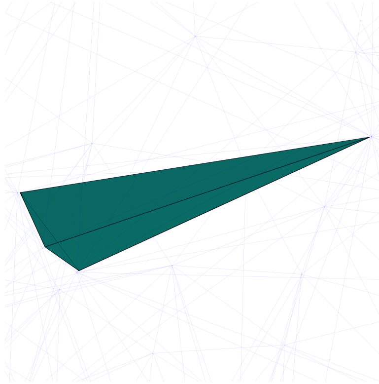
Figure 1.3 A “Kite” in a Delaunay Tetrahedralization
