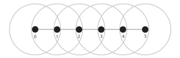
Figure 10: Showing radio range of nodes at power 1 in a single line setup.
