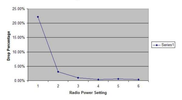
Packet Drop Rate Vs Radio Power
