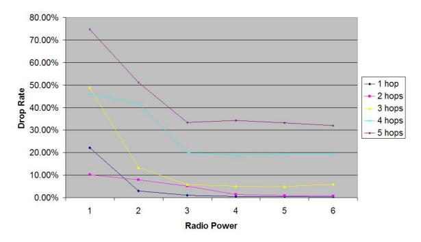
Packet Drop Rate vs Radio Power, Composite
