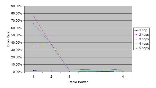
Packet Drop Rate vs Radio Power, Composite
