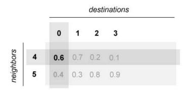
Figure 3: Pheromone table update. As the packet in Figure 2 hops to node 6, node 6 updates its pheromone table to reflect the incoming packet's information. The pheromone table is updated such that neighbor node 4's destination entry for node 0 (source node) has its value adjusted. The rows in node 6's pheromone table reflect the nodes that node 6 can hear locally. The destinations are nodes that node 6 knows about.
