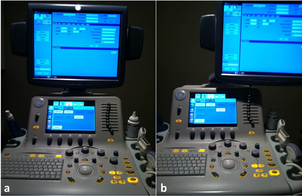
Figure N.8 Monitor in (a) Neutral Arm Position and (b) Extended on the Swing Arm of the Ultrasound System for Alignment with Sonographer's Neutral Line of Sight
