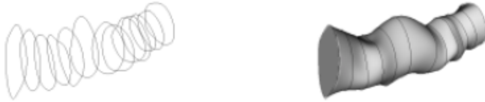
Figure 2.1 Analytic model of a vessel made by lofting surfaces through contours [Wang, 2001]
