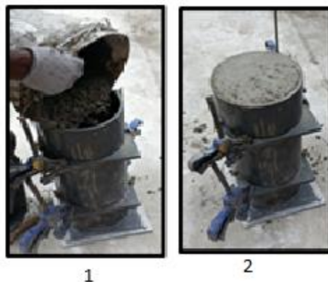
Figure 4.7 The static column segregation
