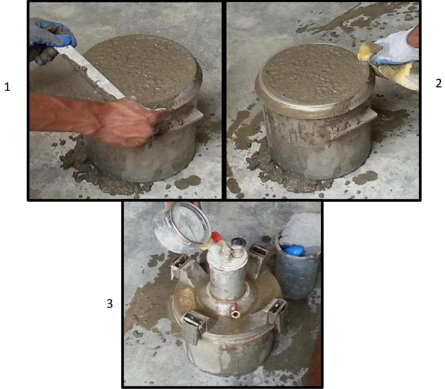
Figure 4.8 Air content test
