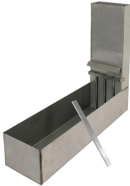
Figure 2.4 L-Box testing apparatus
