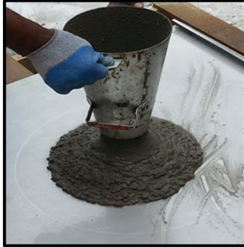
Figure 2.1 Slump flow test
