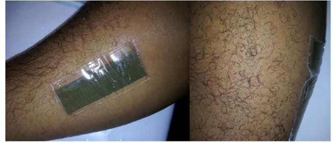
FIGURE 13 Transfer tattoo tag showing air gap after shower test
