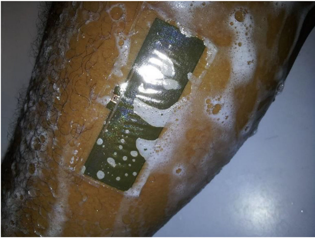
FIGURE 11 Transfer tattoo tag covered with soap during shower test
