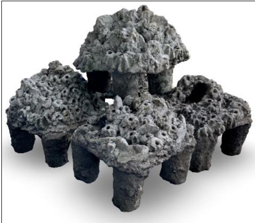
227 228 229 230 231 232 233 234 235 236 237 238 239 240 241 242 243 244 245 246 247 248 Figure 3: 3D model of a set of 5 standard ‘roti buaya’ artificial reef structures, in the stacking 249 configuration commonly used by both NGOs. Model created using Metascan Photogrammetry .
