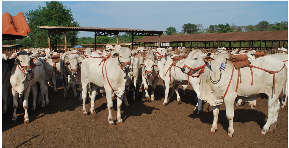
Fig 1. Animals, in a test group, with the apparatus (halter, saddle and cylinder) for methane collection by sulfur hexafluoride (SF 6 ) tracer gas technique.
