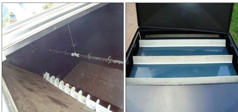
Figure 3: Top view of the helical conveyor and part of the aeration system (on the left) and surface scraper of the Central Unit (on the right) of the Pilot Plant.
