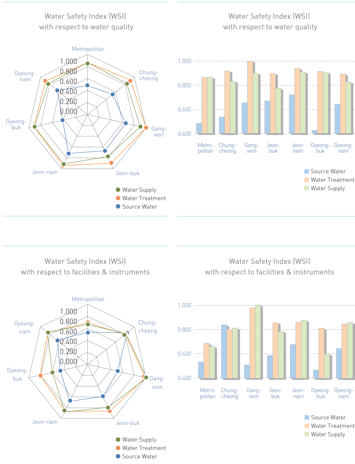
Figure 10b. Water Safety Index (WSI) values for rated water systems based on three water supply process steps and three categories of conditions (water quality, facilities and instruments and maintenance and operation)
