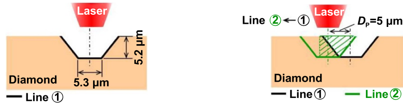
(a) Shape of micro-groove by the first scanning line. (b) Assumed removal region by the second scanning line.
