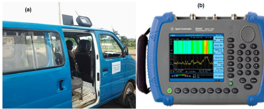
Figure 2. Measurement equipment (a) measurement bus (b) agilent N9342C agilent spectrum analyzer.
