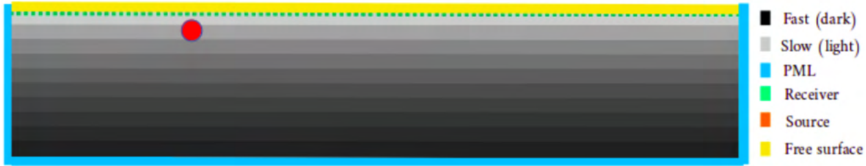
Figure 3.18: Configuration of the computational domain for the 10-layer unconsolidated granular media model.
