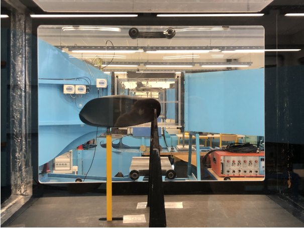
Figure 3: Experimental wind tunnel setup using 3D printed and smoothed BV4 shape.
