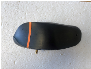
Figure 6: Location of the trip position. Tripping was implemented by employing a sufficiently thin tape wrapped around the shape.
