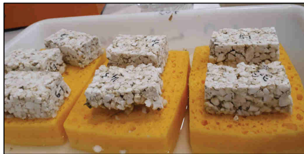
Fig. 1: Capillary absorption test
