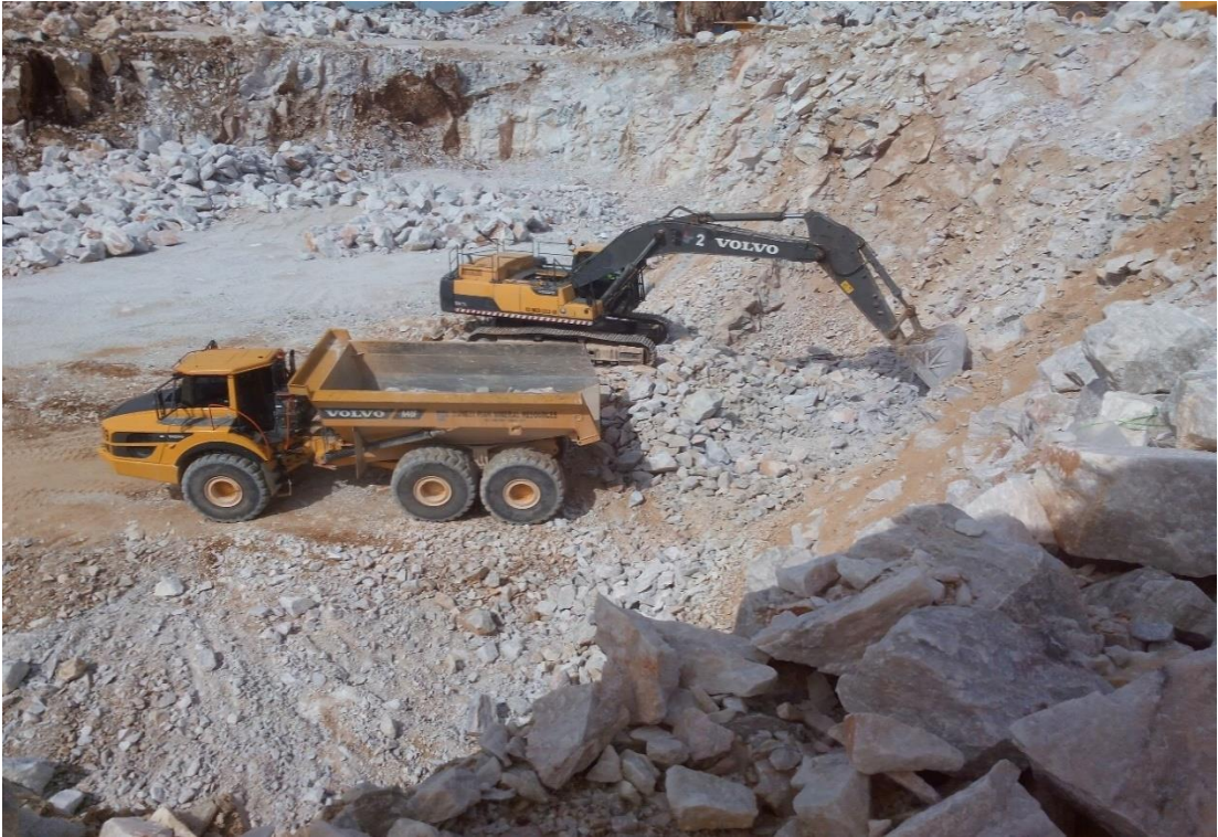
Figure 3.2: Excavator are loading the material into the truck bucket
