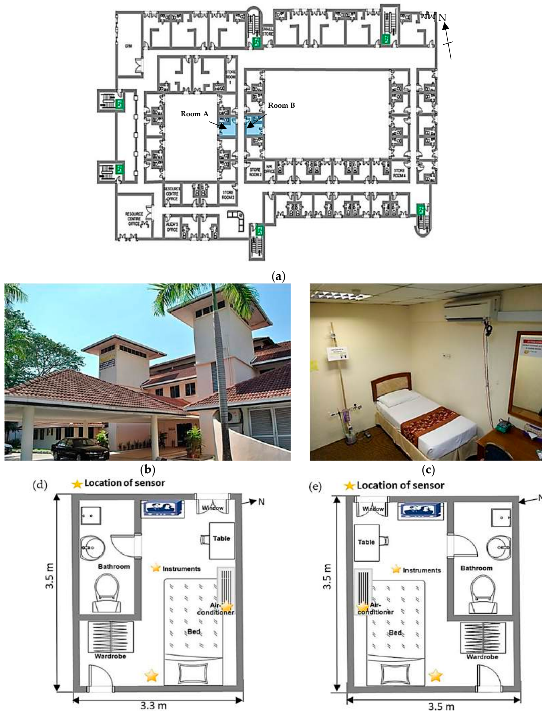
Figure 1. Details of the measurement site: (a) the floor plan of the second floor of the BATC building with the locations of the investigated rooms; (b) the BATC building; (c) an example of the sensor setup in the room; (d,e) the layouts of the investigated rooms A and B, respectively, and (e).
