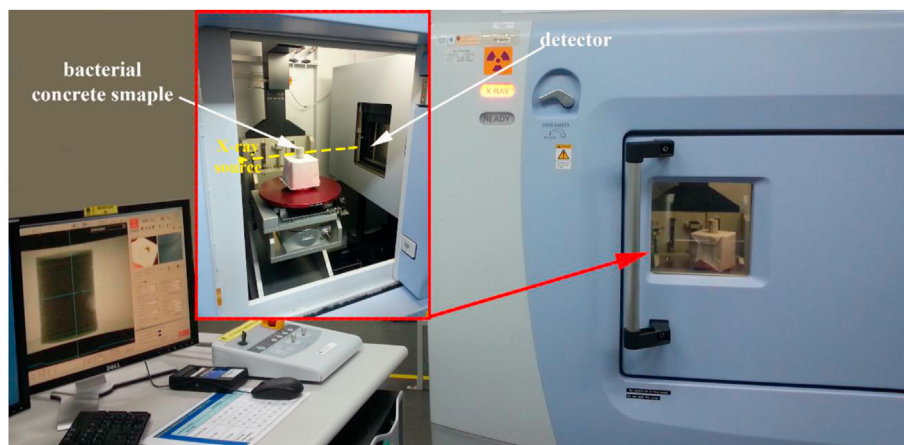
Fig. 1 – X rays CT test for bacterial mortar sample.
